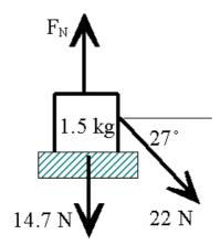
Ex 3:For the mass shown below, calculate the horizontal acceleration and the normal force,  $F_{N}$
