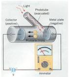
A metal plate and a smaller electrode (collector), are placed inside an evacuated glass tube called a photocell. The metal plate and collector are connected to an ammeter and to a voltage source. The ammeter will read zero when the photocell is in the dark, indicating that no current is present. But when light of sufficiently high frequency is shone on
