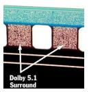
An LED is shone through this pattern as the film passes through the projector. On the other side of the film the light does not hit a photocell but a charge coupled device, and is finally interpreted as an audio signal.
