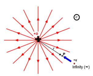
An electron will gain EPE as work is done to force it away from the positive charge
