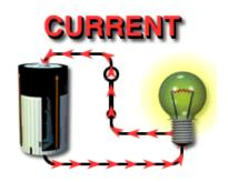
Current is the flow of charged particles along a closed path.
